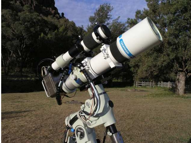
Monte Willsin's prototype 19 th magnitude guide scope, showing the tubes which circulate the chilled surgical alcohol
